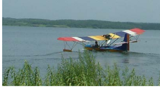
Fig 15 Turning on water within small radius only using air rudder in propeller slipstream
