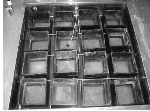
Fig. 2 – Freeze-thaw tests of concrete specimens.
