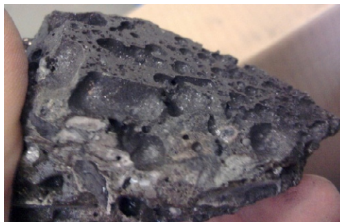
Fig. 7. Slag from plasma reactor after processing the printed circuit boards waste
