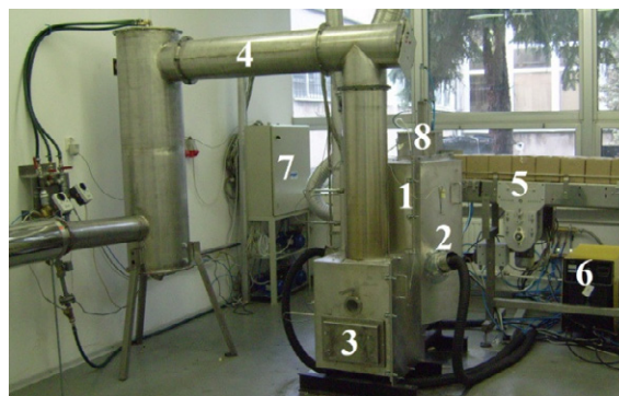
Fig. 2. Overview of the laboratory setup: 1) Plasma reactor, 2) Plasmatron, 3) Molten product collection, 4) Fumes Exhaust – chimney, 5) Waste package transporter, 6) Plasmatron power supply, 7) PLC – automation and data collection apparatus cabinet, 8) Automatic waste package feeder
