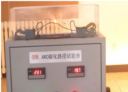
Fig. 4 Serial Arc Test Picture, Resistive Load, Carbonized Route
