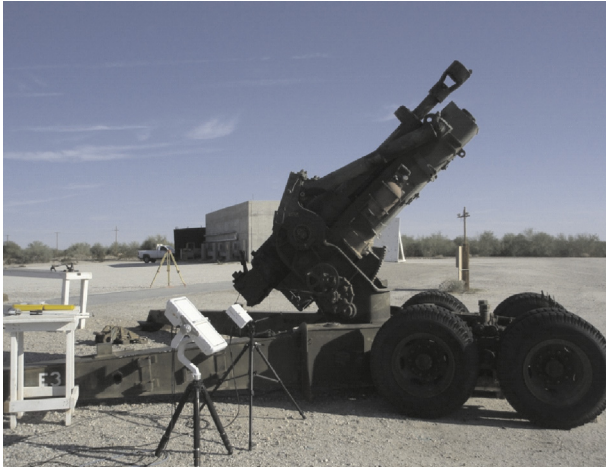
Fig. 5. 105 mm howitzer quadrant elevation set for maximum range.
