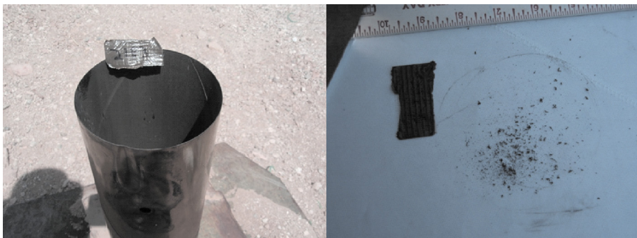
Fig. 15. Sample M1 cartridge case and residue after firing.
