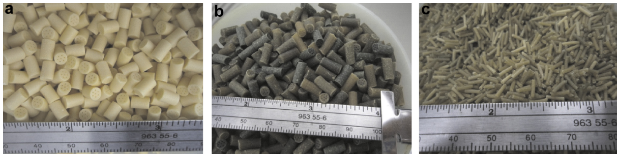
Fig. 3. (a) PAP-029 in seven perforated grain geometry ARDEC Lot RDD13F-00136. (b) M1 seven perforated geometry Lot RAD11C-071981. (c) M1 propellant in single perforated geometry Lot RAD11C-071984.
