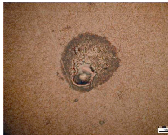
Fig. 3: View of a crater produced at the surface by the spark. Melted material can be seen [2].
