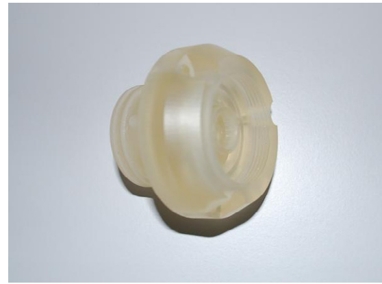
Fig. 14: Rapid prototyping nozzle used for tests.
