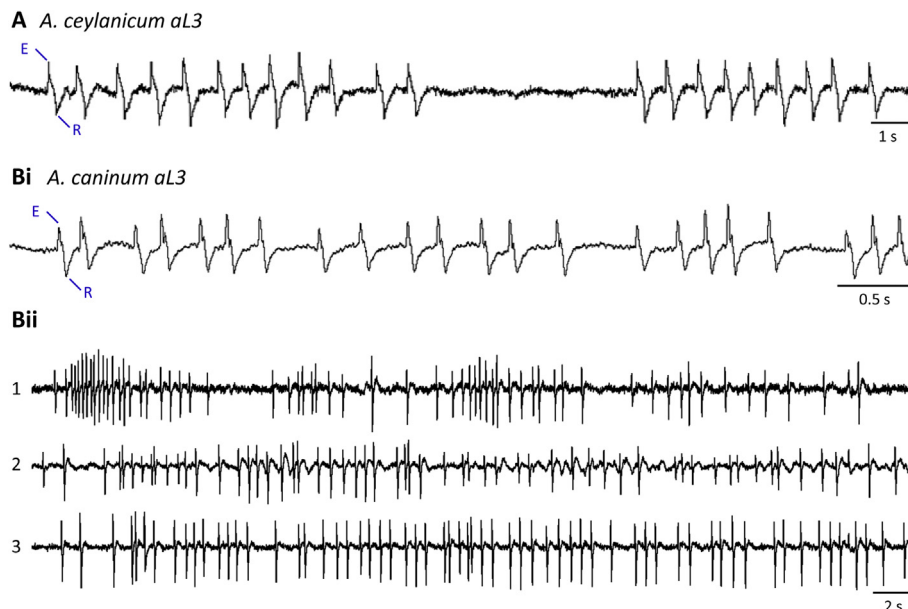
Fig. 2. Microfluidic EPG recordings from activated L3 (aL3) hookworms. A. A. ceylanicum aL3s, in M9 with 15% HS and 10 mM 5HT, 28 °C. E and R spikes in the pump waveform are marked in A and Bi. B. A. caninum aL3s. i. In M9 with 1 mM 5HT, 38 °C. ii. Three worms in one chip (numbered 1 to 3; each trace from a different worm), in M9 with 5 mM 5HT, 42 °C. All worms were recorded 1 d after in vitro activation.
