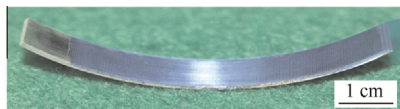
Fig. 13 Patterned dry-film photoresist with through-holes 50 \mu\text{m} in diameter coated onto a cylindrical inner surface.
