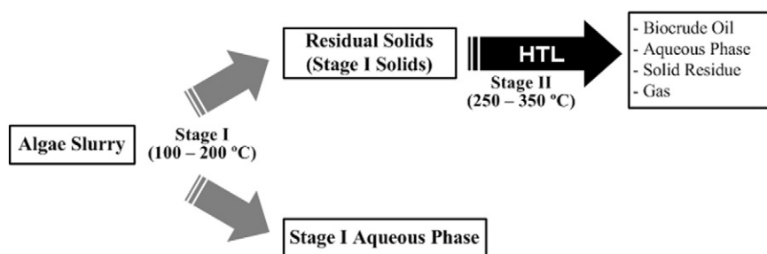
Fig. 1. Schematic diagram of the two-step hydrothermal liquefaction process.
