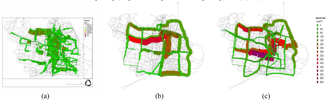
Fig. 11. Load public transport networks in the current trend 2030 (11a) and in the alternatives (BRT-grid structure (11b), and PT-system (11c))
