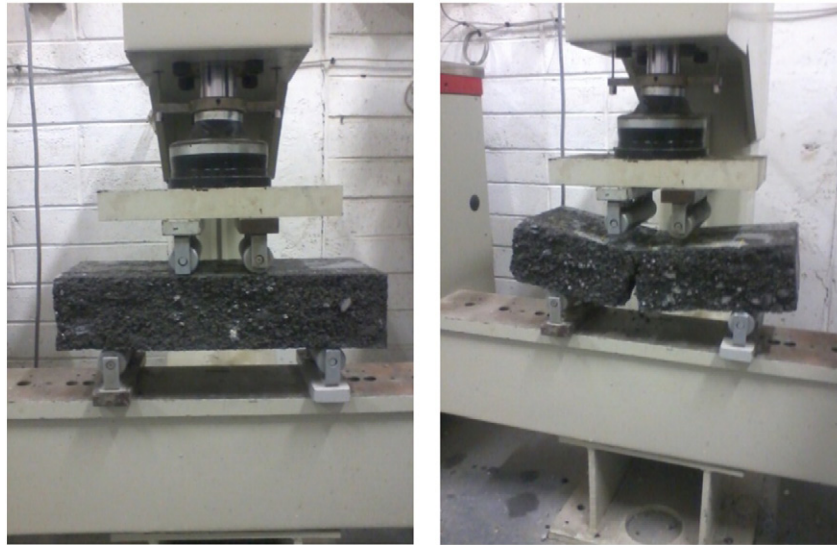
Fig. 3. Masonry block undergoing flexural loading.
