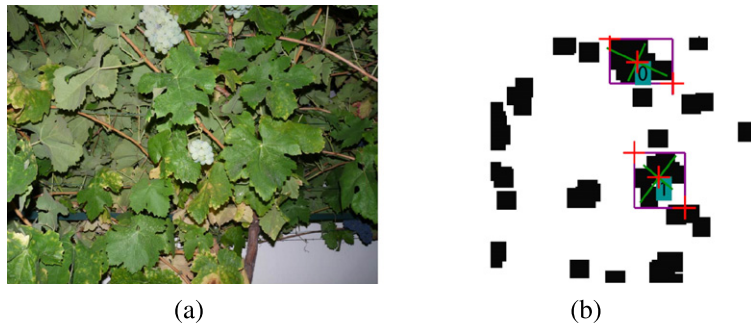
Fig. 4. Example of a possible robot's positioning correction by noticing "how far" it is from the bunches: (a) original image; (b) identification result.
