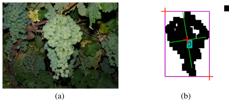
Fig. 6. Example of a possible robot's positioning correction by noticing the presence of more bunches; (a) original image; (b) in this case, only the central bunch was correctly identified, so more pictures are needed (see text).
