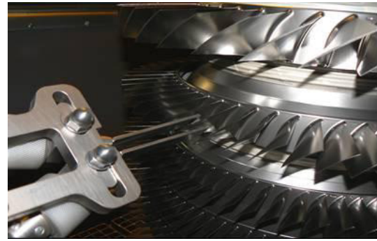
Fig.8: Peening of a 4 stage blisk rotor [1]
