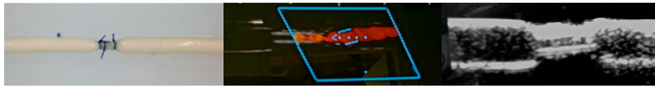
Fig 2. A , Ovine artery with snares to fix stenosis tube. B , Flow velocity measurement by duplex ultrasound (DUS), proximal to stenosis tube. C , B-mode ultrasound image of stenosis tube.
