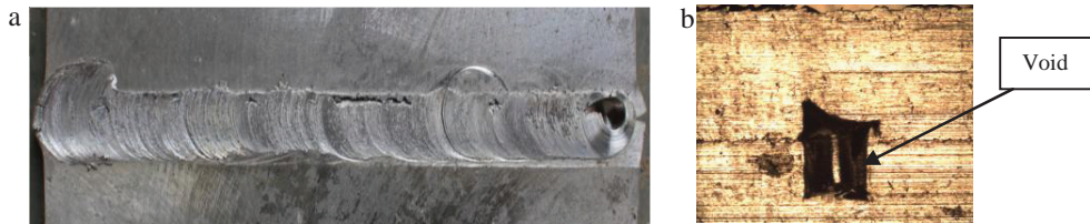
Fig. 10. Experiment 8 (a) weld pool close view; (b) microscopic view (100X).
