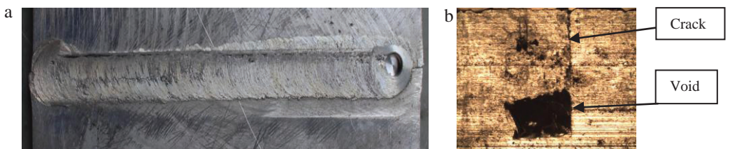
Fig. 9. Experiment 7 (a) weld pool close view; (b) microscopic view (100X).
