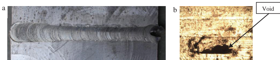
Fig. 3. Experiment 1 (a) weld pool close view; (b) microscopic view (100X).
