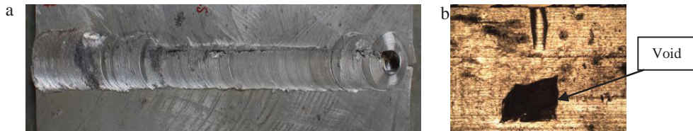
Fig. 11. Experiment 9 (a) weld pool close view; (b) microscopic view (100X).
