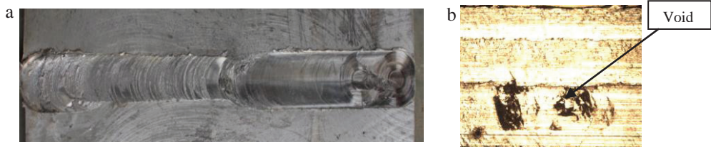
Fig. 4. Experiment 2 (a) weld pool close view; (b) microscopic view (100X).
