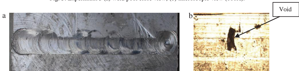
Fig. 6. Experiment 4 (a) weld pool close view; (b) microscopic view (100X).
