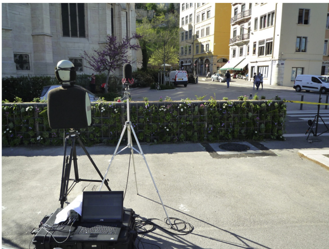
Fig. 7. Low height vegetated barrier along a road with head-and-torso simulator behind the barrier for acoustic recordings [103].
