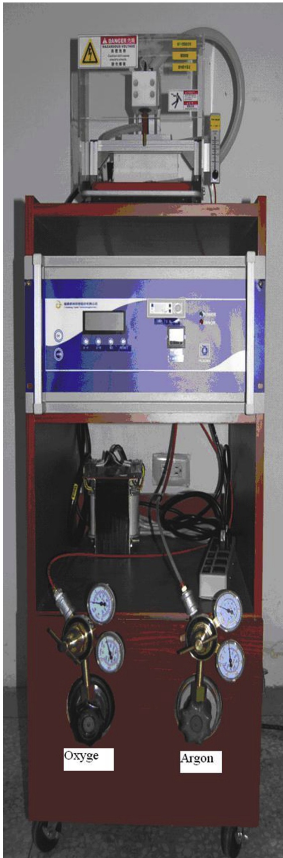
Fig. 2. Non-thermal dielectric barrier discharge plasma device manufactured by Taiwan Yih Dar Technologies, Changhua, Taiwan. Aluminum tape
