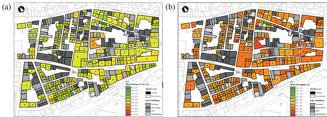
Fig. 4. Damage scenario for I_{(EMS-98)} = VIII (a) and I_{(EMS-98)} = IX (b)
