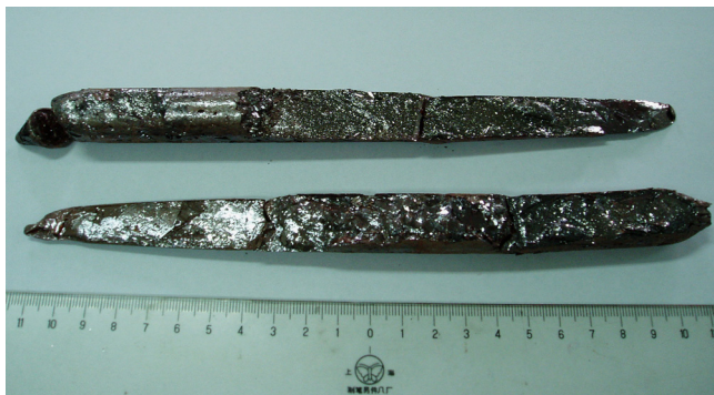
Fig. 1. The photograph of about 200–300 g as synthesized GaSe polycrystals.
