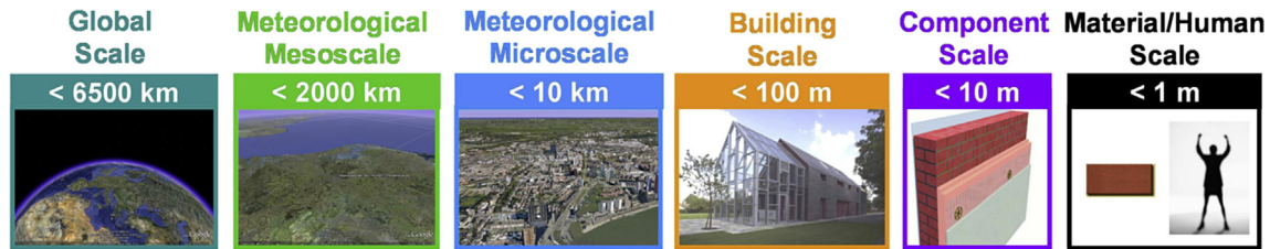
Fig. 2. Schematic representation of relevant spatial scales in pollutant dispersion. From Blocken et al. (2013).
