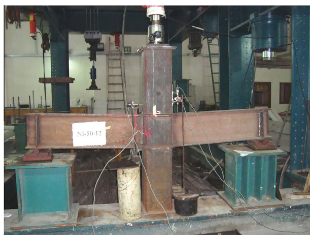
Fig. 8 Deformed shape during test for specimen NI-50-12.
