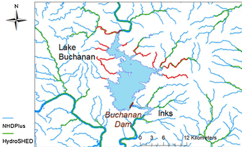
Fig. 5. NHDPlus river network as RAPID model baselines: 14 inflows are marked in red.
