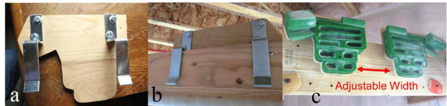
Fig. 7. Adjustable hangboard mount. (a) rear view showing brackets that fit over and slide across a 2”x10” beam. (b) adjustable mount in use on the beam, from the rear, and (c) from the front.
