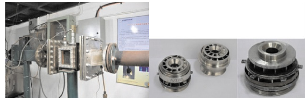
Fig. 1 LBO test rig and dual-axial/axial-radial/dual-radial swirl-cup assemblies.
