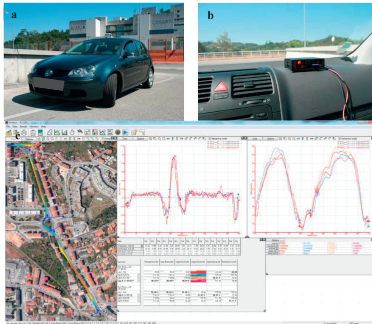
Fig. 3. Data collection: (a) Instrumented vehicle; (b) Data logger DL1 MK3 equipment; (c) Race Technology software – data output.
