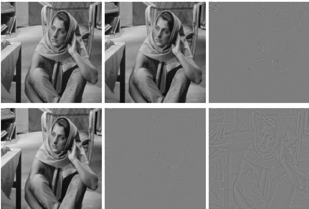
Fig. 5. Top from left to right: initial woman image f , \tilde{u} , and \tilde{v} + 150 , computed with Db10 (Method C), \alpha = 0.5 , \gamma = 0.002 ; bottom from left to right: u and v obtained by the Vese–Osher TV model and the v component obtained by the Vese–Solé–Osher H^{-1} model.
