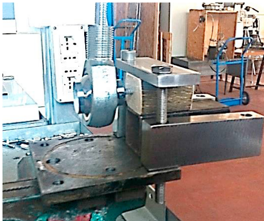
Fig. 8. Experimental setup of bending fatigue tests.
