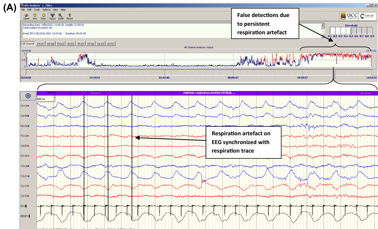
Fig. 10. Causes of false detection. (A) Respiration artefact. Upper panel shows output from SDA, lower panel shows rhythmic respiration artefact on EEG synchronized with respiration trace (from motion sensor). (B) Pulse artefact synchronized to ECG trace. (C) Sweat artefact with characteristic high amplitude semi-rhythmic slow waves spanning several seconds. (D) Highly rhythmic background EEG occurring in the intermediate sleep phase. Note how periodic episodes of intermediate/quiet sleep indicated by the CFM are coincident with periods of raised seizure probability output on the SDA graph and a highly rhythmic EEG in the lower panel.
