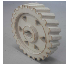
Fig.2 Formed helical gear of WPC ( D_2=79.85\text{mm} , b_2=19.73\text{mm} )
