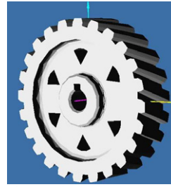
Fig.1 Helical gear three-dimensional model ( D_1=80\text{mm} , b_1=20\text{mm} )
