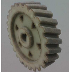
Fig.3 Formed part after post-processing ( D_3=79.25 mm, b_3=19.52 mm)
