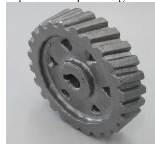
Fig.8 Investment casting gear ( D_1=78.41\text{mm} , b_1=19.66\text{mm} )
