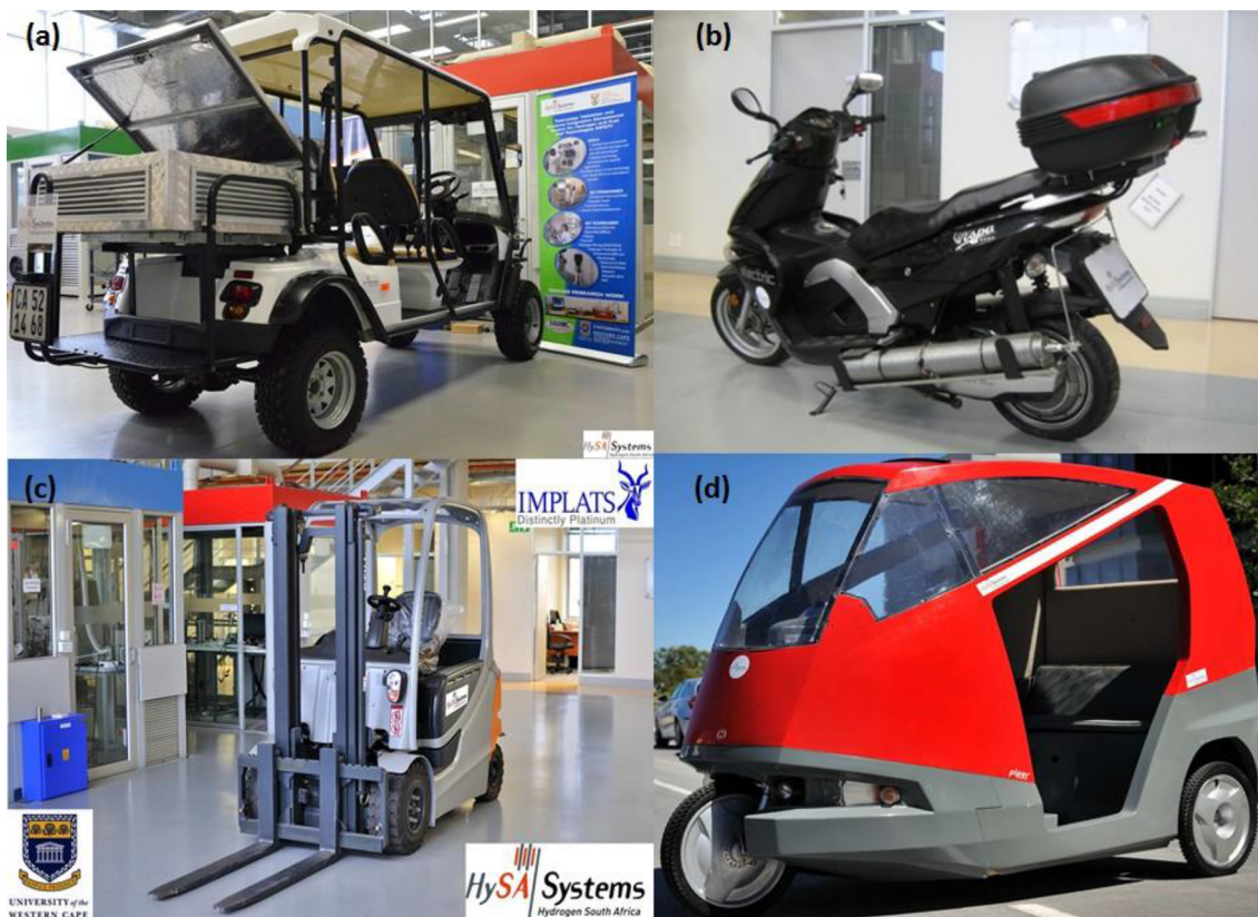
Fig. 20 – Fuel cell powered vehicles at HySA Systems: (a) golf cart (Melex), (b) e-scooter (Melex), (c) forklift (STILL International), (d) three-wheeler (Microcab).
