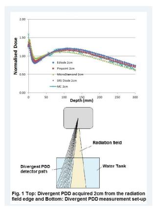
This results in a Dmin occurring out-of-field at approx. the same depth where Dmax occurs in-field. However at 15cm from the field edge the second build-up region disappears for all detectors. The measured divergent PDDs agree to within 0.5% of each other over the range of out-of-field distances examined. Initial comparison to MC reveal good agreement however the MC PDDs have a large statistical uncertainty.
