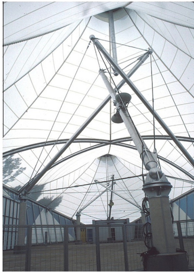
Fig. 12. A full-scale model serving for the skeleton of a membrane structure in Chiba Japan.
