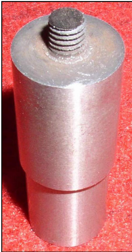
Fig. 4. Fabricated friction stir processing tool.
