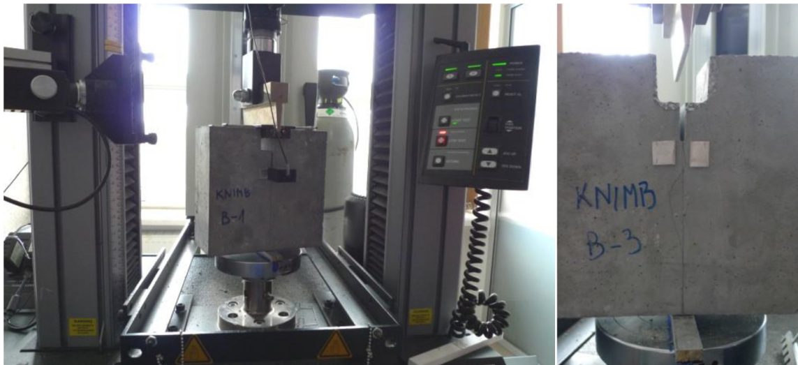
Fig. 2. Experimental setup of the wedge splitting test.
