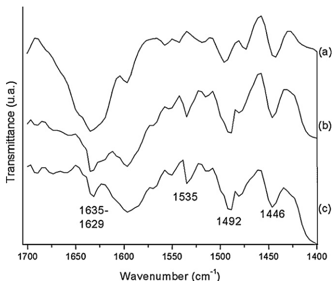
Fig. 7. IR spectra in the region 1700–1400 cm -1 of MF9S4 (a) without adsorbed pyridine and (b) with adsorbed.
