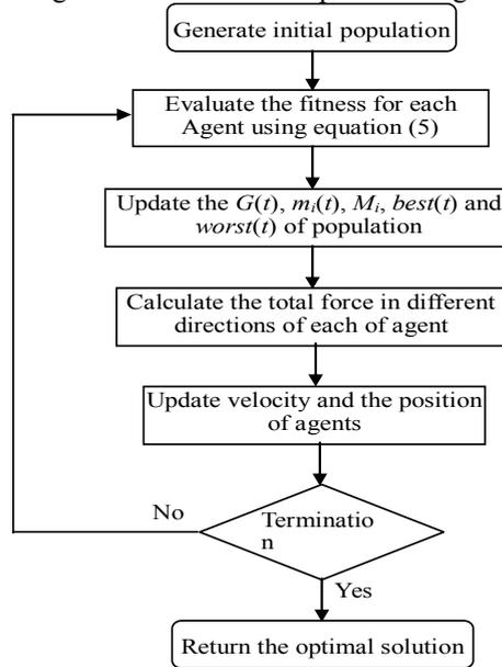
Fig. 2. Flowchart diagram of GSA for grey image enhancement
