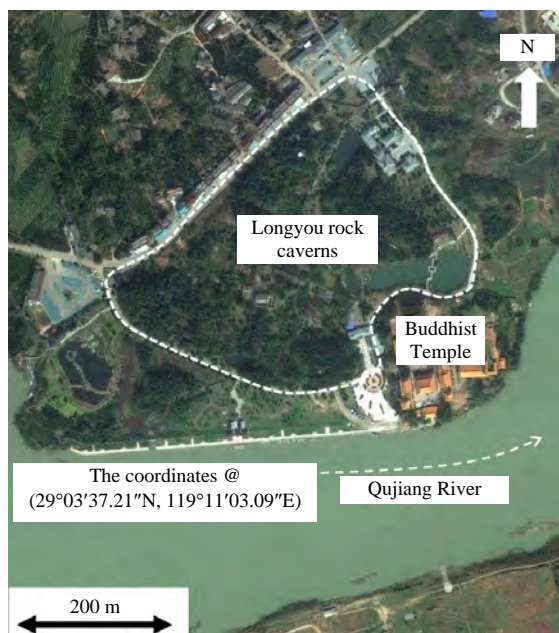
Fig.2 Longyou rock caverns in a small hill with uneven ground elevations of 47 to 60 m, and comprising argillaceous siltstone of Cretaceous age on northern bank of Qujiang River with elevation of 36 m near Longyou County (drawn on satellite image of Google Map 2011).
