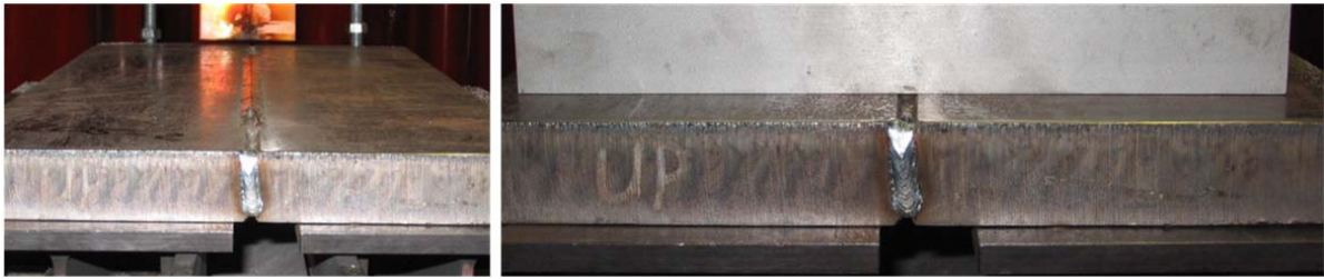
Fig. 4. X65 pipeline steel, 35 mm wall thickness – remaining thermal distortion after double-sided, single pass connection weld.
