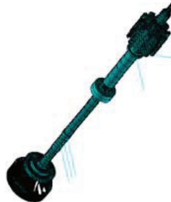
Fig.2 The finite element model of the main shaft system
