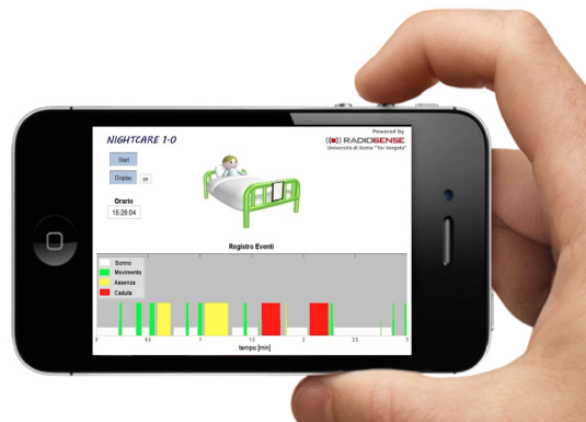
Fig. 6 Real-time visualization of the NightCare system on mobile platform
