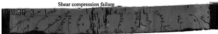
Fig. 4. Mode III failure: crushing of the concrete in the shear compression zone.
