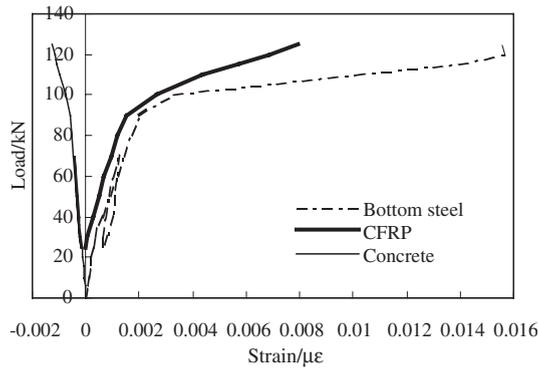
Fig. 12. Load–strain curves of CFRP, bottom steel and top concrete for beam RDBL30-1A.
