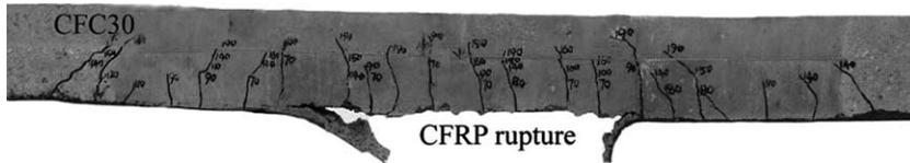
Fig. 3. Mode II failure: rupture of CFRP.
