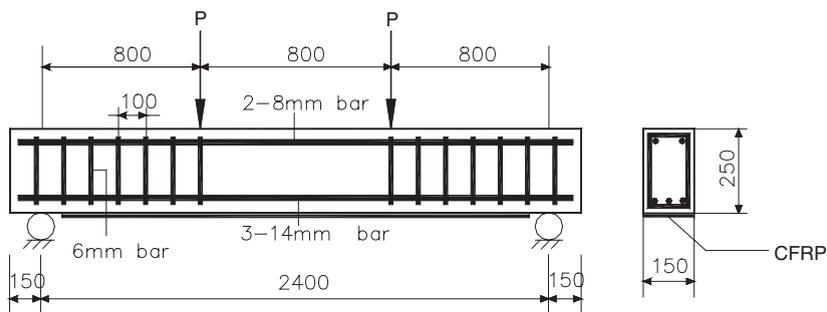
Fig. 1. Details of test beams (dimensions in mm).
