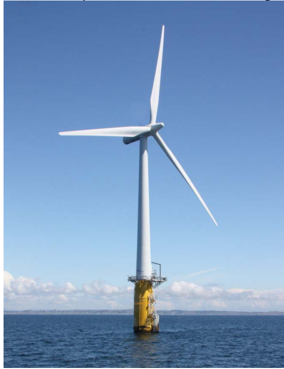
Fig. 1. Statoil's Hywind Demo floating offshore wind turbine utilizing a Siemens' 2.3-MW Turbine with an 82.4-m rotor diameter.
