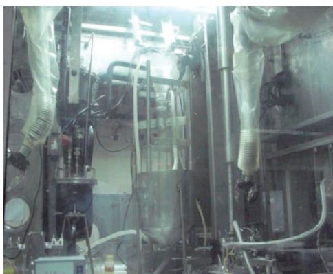
Fig.1. Gelation setup comprising glass column with silicone oil and other equipments inside glove box
