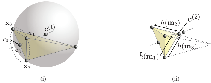
Fig. 4. Placement of off-centre Steiner points in the volume \Omega , showing (i) the local edge v_e \in \text{Vor}(X) of the Voronoi diagram associated with the small face f_0 \in \tau , and (ii) placement of the size-optimal vertex \mathbf{c}^{(2)} , such that local size constraints \bar{h}(\mathbf{x}_\tau) are enforced.
