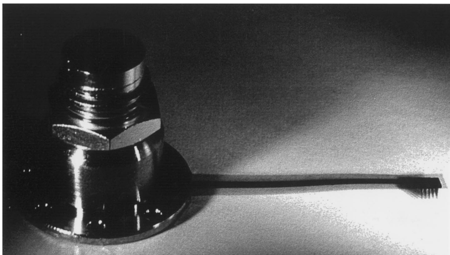
Fig. 3. A photograph of a chronic 25 electrode, UEA assembly that uses a 20 micron thick, polyimide ribbon cable to connect the array to a transdermal connector.
