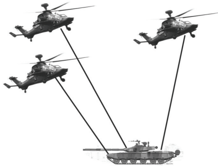
Fig.1 Suspending and carrying model of close-coupling multiple helicopters system.
