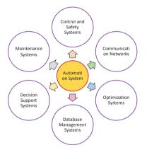
Fig. 6. Functional sub-systems of a smart grid system.
