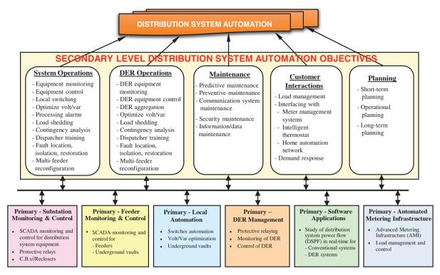
Fig. 5. Primary level and secondary level objectives of power distribution system automation.
