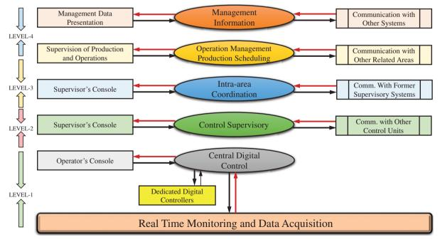
Fig. 3. Functional representation of a generic automated system architecture.
