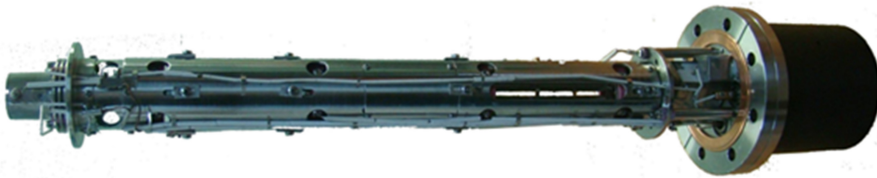
Fig. 2. Five-section quadrupole Paul trap of linear configuration with energy filter and ion source.
