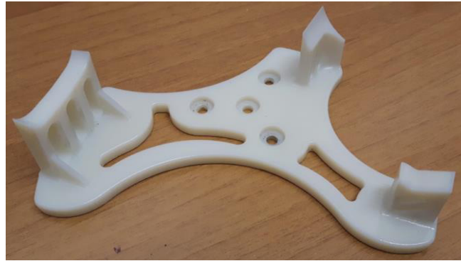
Fig. 8. Final fixture made by additive manufacturing
