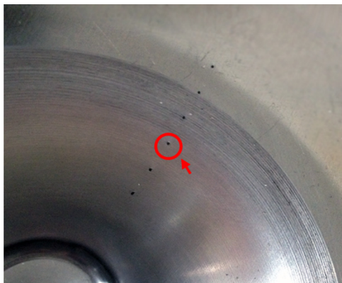
Fig. 20. Hyperbolic cone with small holes. (For interpretation of the references to color in this figure, the reader is referred to the web version of this article.)
